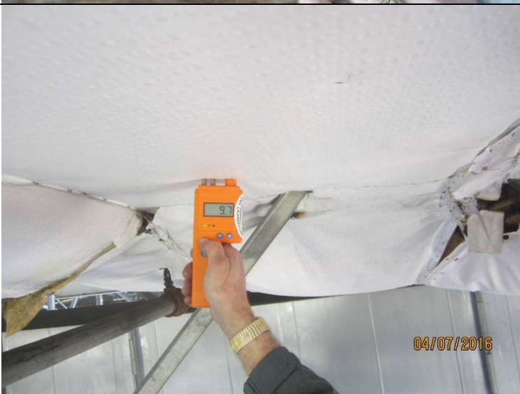
Photograph 27: Delmhorst reading indicating low moisture.
