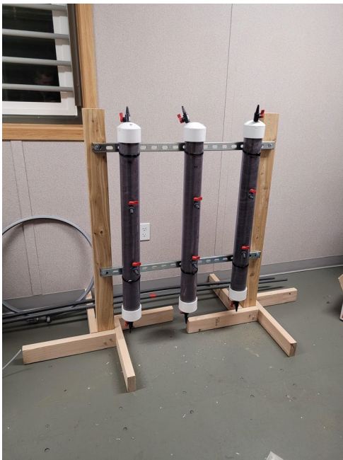
Photograph 2. Flow-through column setup
