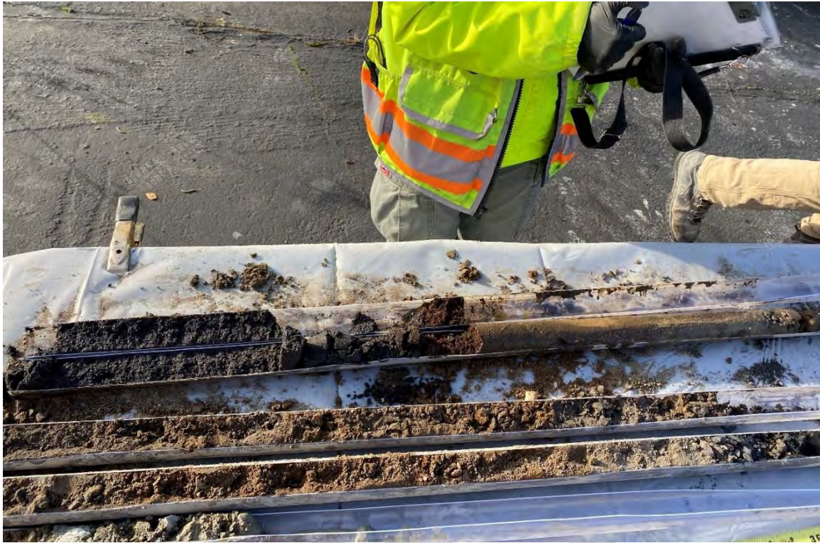
Figure 10. Core taken from AB-1, 15-20 fbs (top). Note transition from sandy silt (right) to coarse dark sand (left).
