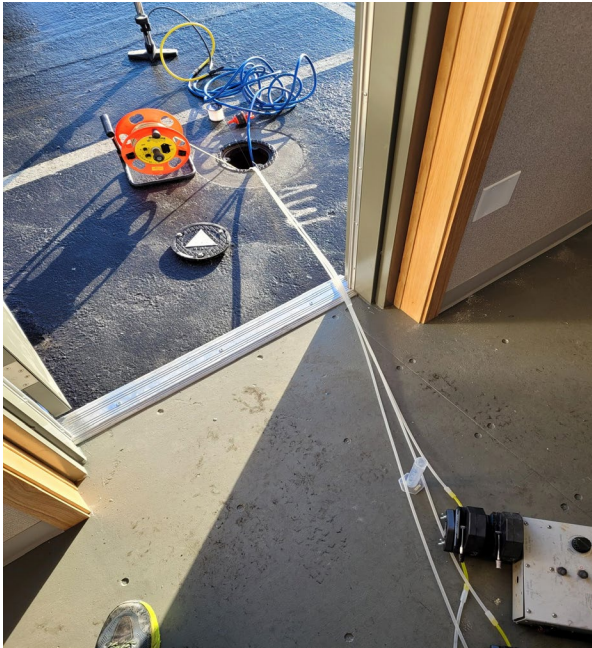
Photograph 1. MW-14 well head with pump tubing (x3), inflatable packer, and water level meter.
