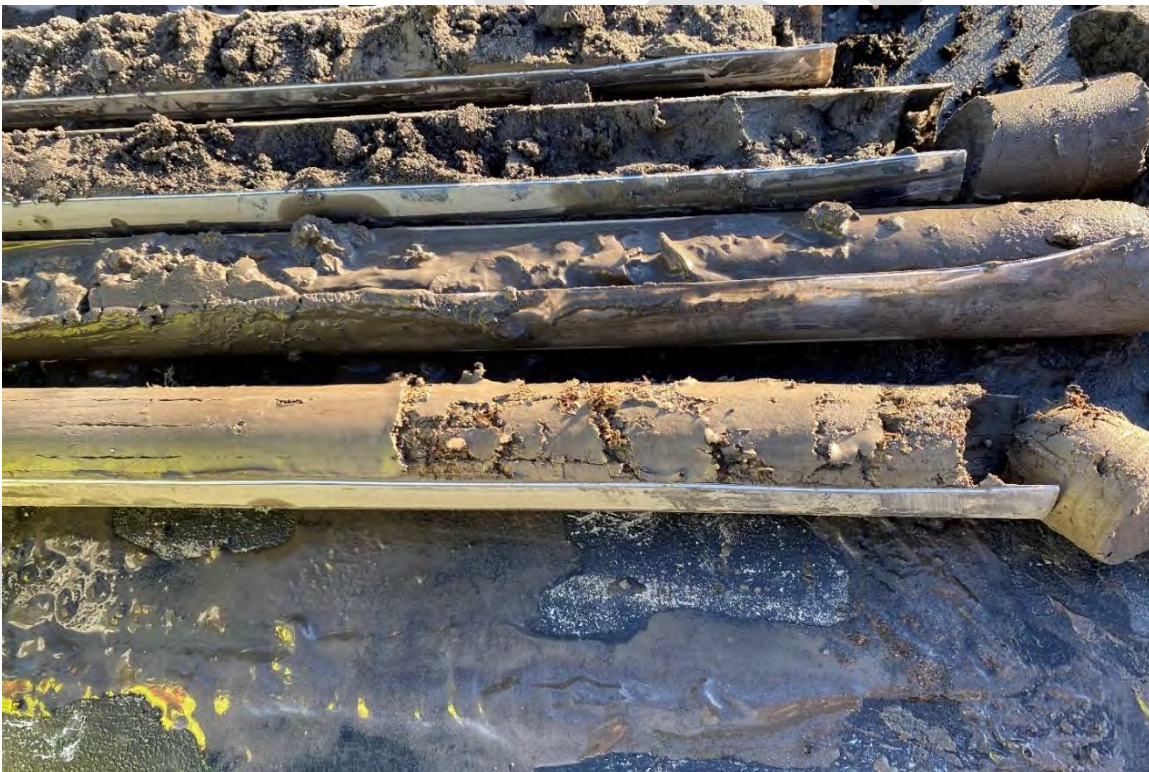
Figure 9. Woody debris in AB-4, from approximately 24.5-25 fbs.
