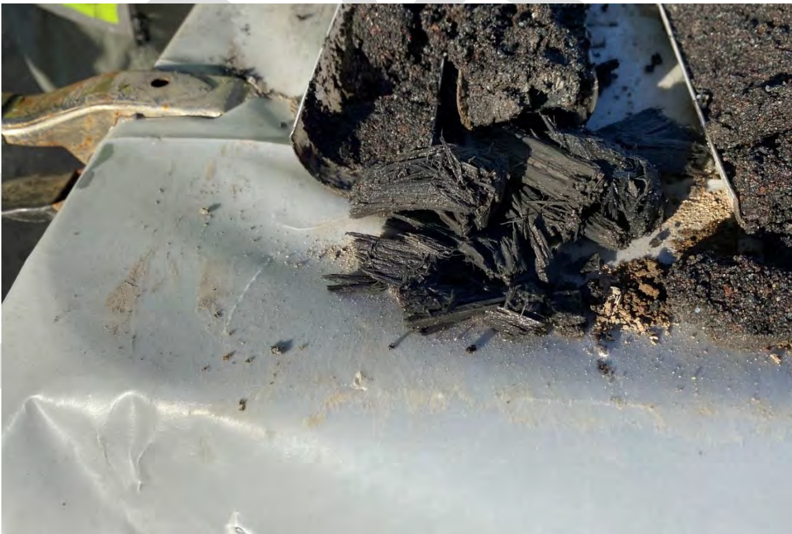
Figure 11. Wood debris from AB-1, taken from bottom of probe at 25 fbs.
