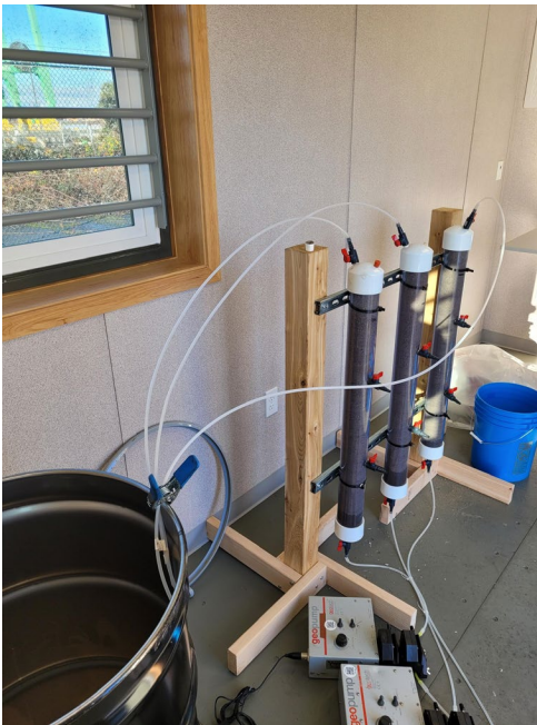
Photograph 4. Flowing columns and effluent discharge.
